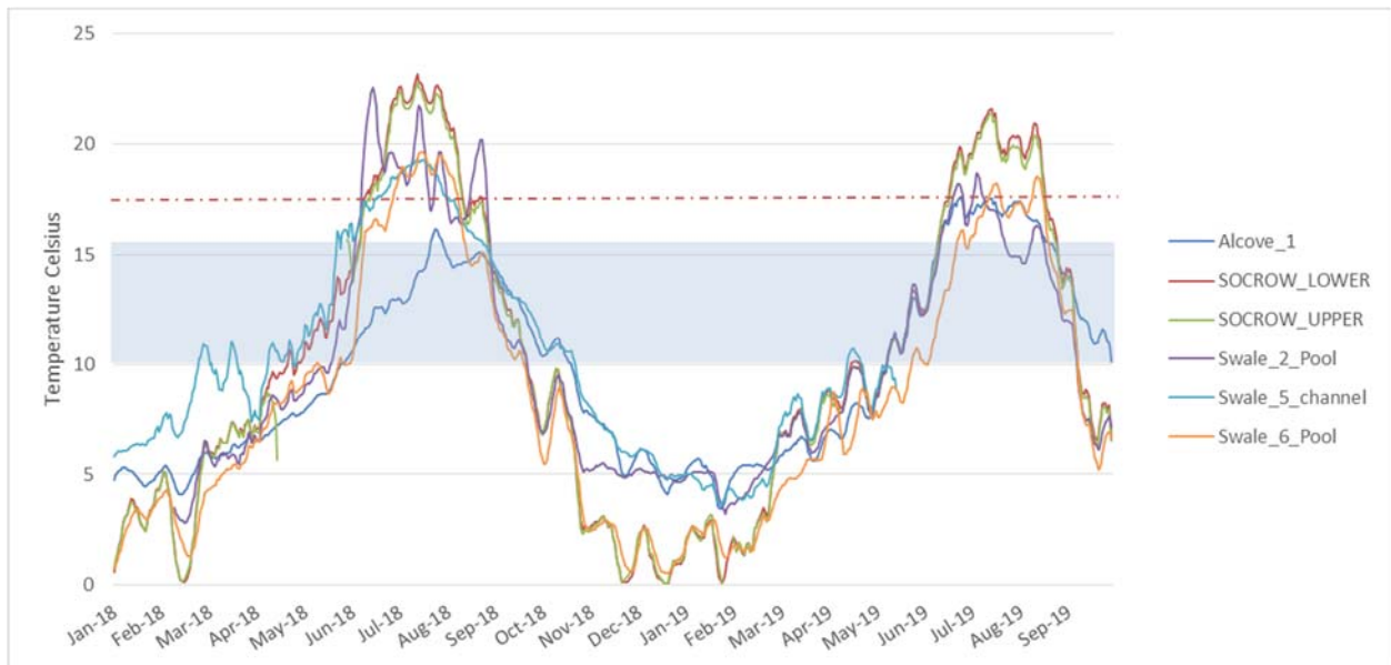
FIGURE 64 7 DAY AVERAGE DAILY MAXIMUM STREAM TEMPERATURE IN CATHERINE CREEK MAINSTEM (RED) AND FLOODPLAIN FEATURES (BLUE) FOR YEARS 2018-2019. NOTE STREAM TEMPERATURE ATTENUATION IN FLOODPLAIN FEATURES DURING SUMMER PEAK TEMPERATURES AND WARMER TEMPERATURES DURING WINTER. . BLUE BOX IS OPTIMUM FEEDING TEMPERATURES FOR JUVENILE CHINOOK (10-15.6°C) AND RED DASHED LINE IS UPPER LIMIT FOR CORE JUVENILE REARING
